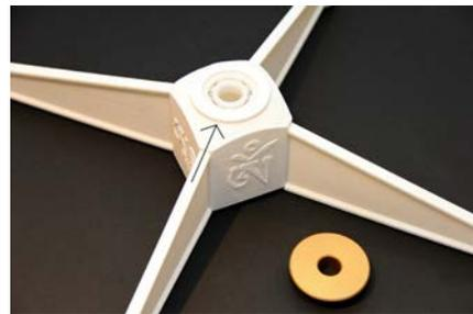
4. Insert the 1.375" white circular ball bearing in the top of the center base so that you can see the circle of small stainless steel ball bearings (i.e., facing up).
